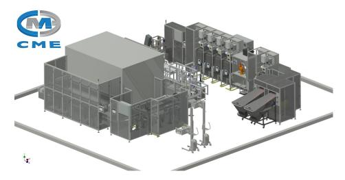
CME's contribution to this prestigious project began when the company secured an initial contract for the design element of a complete bespoke system capable of receiving on-demand orders, filling pill bottles with the appropriate number of tablets or capsules of the requisite drug, labelling bottles and consolidating those orders all whilst ensuring full product tracking and traceability.
